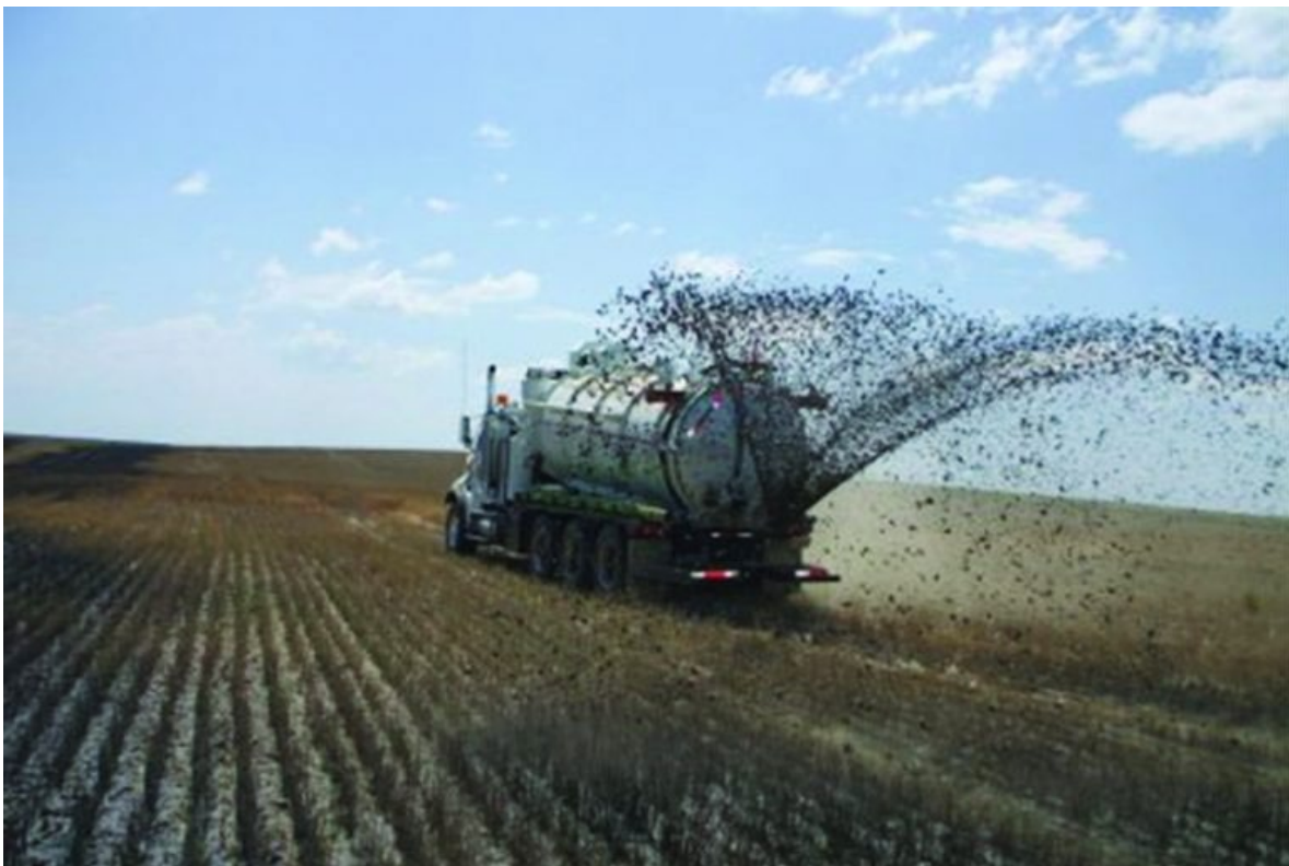
Figure 4 to spread waste faster, tanker trucks like the one pictured replaced ag spreaders
